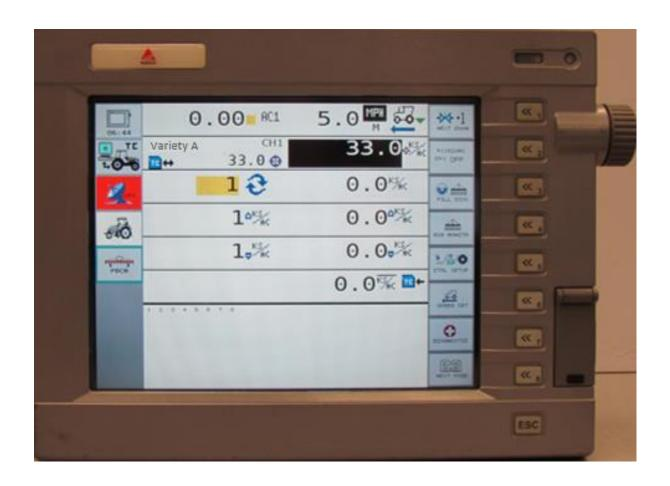
Press the **Task Controller** icon to start a new task. **Note: To switch to a different field the current task must first be ended and steps 1-7 repeated after selecting the new field**
