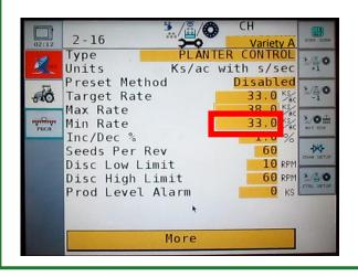
Press the **arrow** to select Planter Control. Press the **check mark** when you finished.
