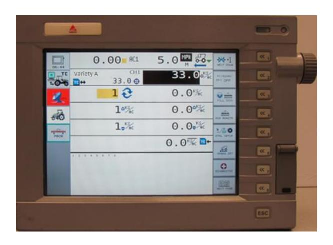
To change products within a Task the current Task must first be stopped. Press the **Stop Light** button to end the Task. **Note:** most prescriptions change rates based on product type.
