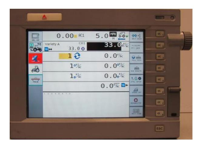
Insert the SD card containing the Task Data and .xml files into the FieldStar II display.
